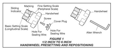
**Step 2.** Turn the handwheel so that the arrow on the sliding indicator matches the basic adjustment value. One complete turn of the handwheel adjusts the indicator one full position.
