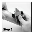
**Step 2.** To assemble the strap on the pipe, remove the "U" bolt. Place the outlet housing over the hole in the pipe. Verify that the housing spike is positioned in the hole.
